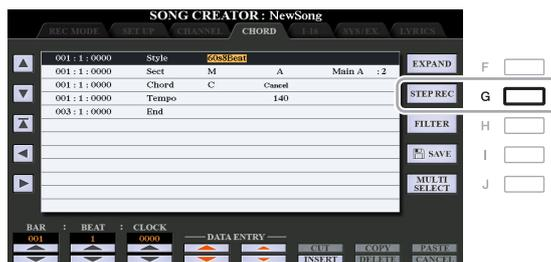
**5 Start Step Recording by using the [A]–[J] buttons and [1 ▲▼]–[8 ▲▼] buttons, as well as the keyboard.**
