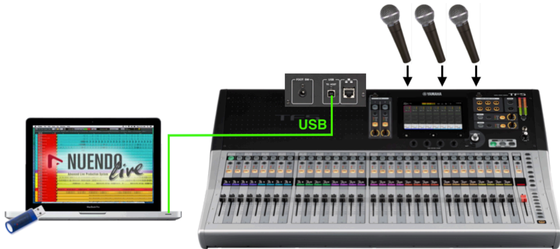
Simple live recording system with TF5
