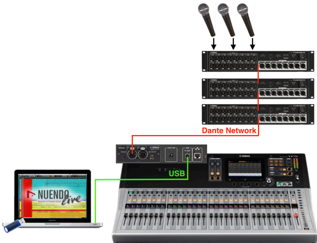
Live Recording system with TF5 & Tio1608-D I/O racks.
