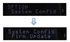
Initially, "Network" is flashing on the display. To perform USB update, select "**USB**" using **UP/DOWN** buttons and press **Enter** button.
