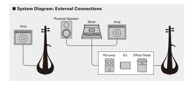
\* The input impedance of the first device (preamp, direct box, etc. ) the instrument connects to has a major influence on the sound quality produced by the speakers. In order to obtain the maximum performance from the instrument, we recommend connecting to a device with an input impedance of more than  $1M\Omega$ .
