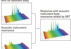
The Yamaha SRT (Studio Response Technology) Powered System is a digital technology that employs in-depth analysis of the acoustic properties of actual musical instruments to add natural-sounding body resonance in real time to instruments such as the SILENT Bass™ that do not have a physical resonant body.
